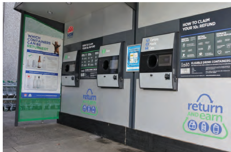
Image: a typical reverse vending machine.
