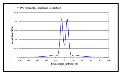
Figure 19 Maximum 11kV overhead line electric field (Source: www.emfs.info/sources/overhead/specific/11-kv)
