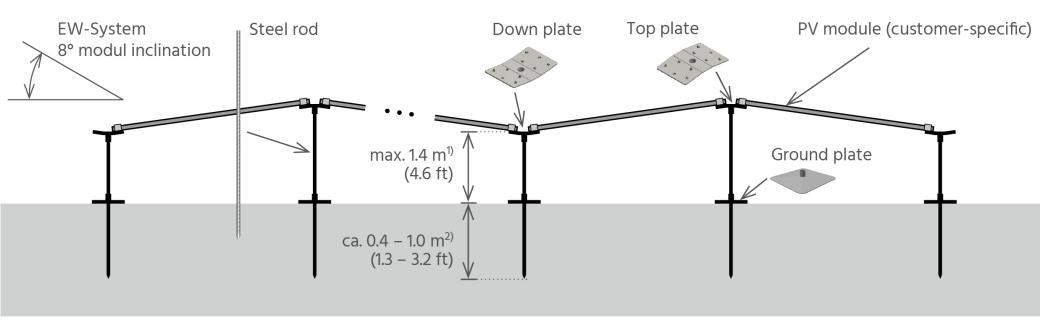
Height Scale Proposed solar array not materially higher than existing farm fence line.
